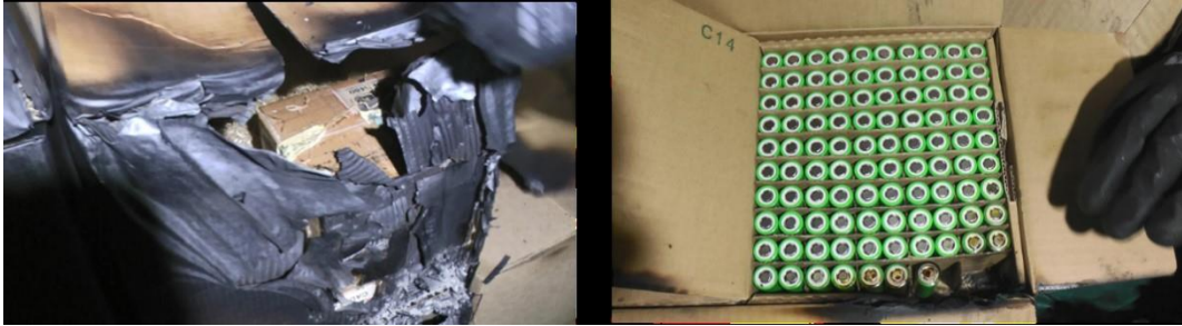
Figure 23: Impact on Cells after the test with Fire Suppression and a Fire Containment Cover.
