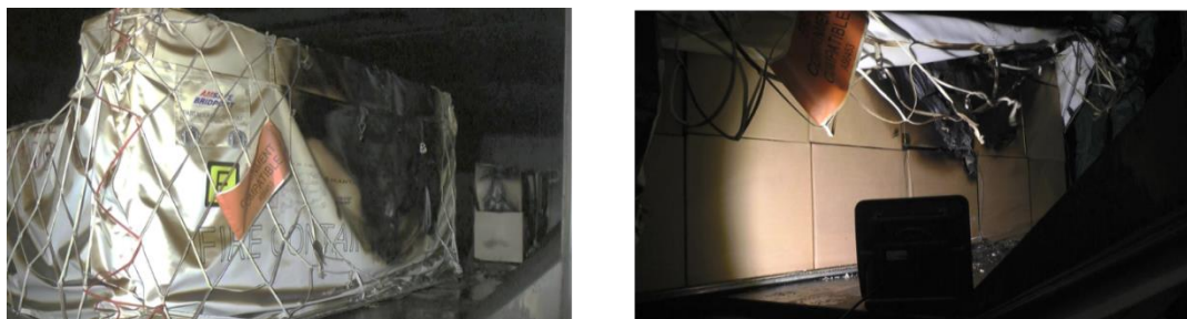
Figure 22: Fire Containment Cover after the test.
