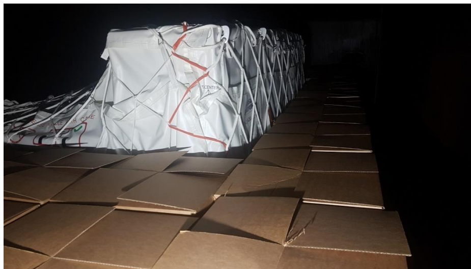
Figure 21: Fire Containment surrounded by fibreboard boxes before the test.
