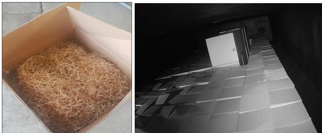
Figure 14: Fibreboard Box filled with shredded paper acting as fire source for the external fire test (left) – Fibreboard Box arrangement in the test compartment (right).
