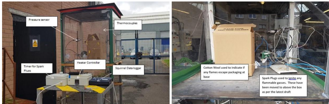
Figure 1: Test chamber constructed to the specifications shown in the AS6413 draft standard.
