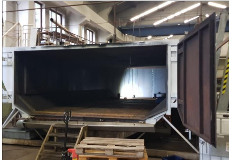
Figure 13: Photograph of the fire test chamber.
