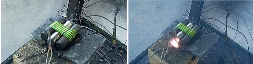
Figure 5: Pictures from the Phase II (Test 16) (left) set-up; (right) during testing showing the heater cartridge becoming detached from the initiation cell.
