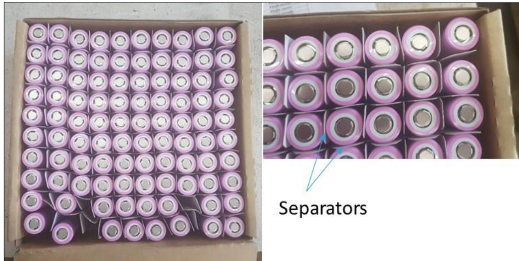
Figure 3: Manufacturer 1 cells packaging (the missing cells were taken to do some voltage checks). On the right a close up picture showing the separation between the cells.
