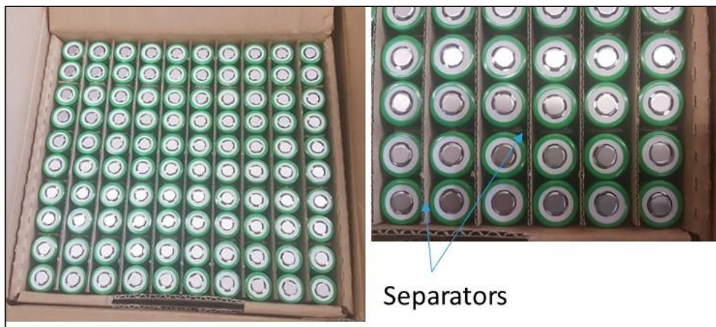
Figure 4: Manufacturer 2 cells packaging. On the right a close up picture showing the separation between the cells.
