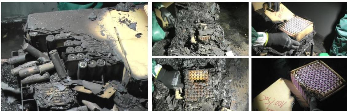
Figure 45: Impact on Cells after the test with fire suppression
