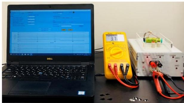
Figure 1. The laptop computer hosts the diagnostic software. The instrument on the right is used to access cell voltage and current in response to discharge or charge profiles applied to the cell (on top of the instrument).
