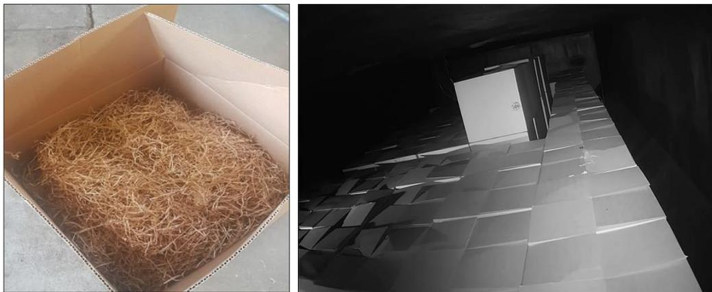
*Figure 36: Cardboard Box filled with shredded paper acting as fire source for the external fire test (left) – Cardboard Box arrangement in the test compartment (right)*
