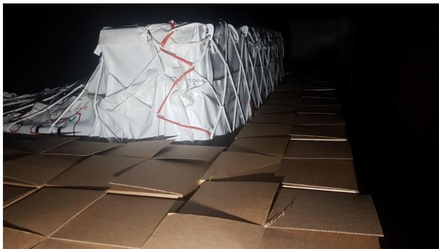
Figure 47: Fire Containment Cover within cardboard boxes before the test
