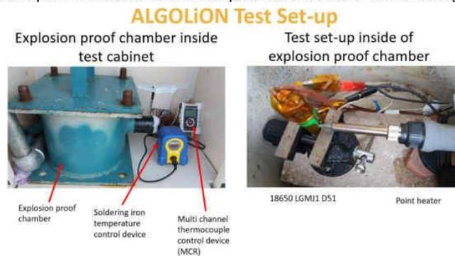
Figure 57: Experimental Setup at ALGOLiON for 1 cell heating temperature measurements
