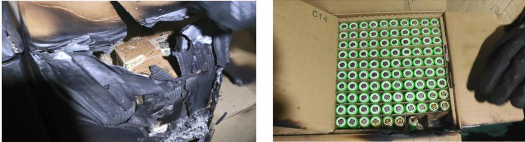
Figure 49: Impact on Cells after the Test with Fire Suppression and Fire Containment Cover
