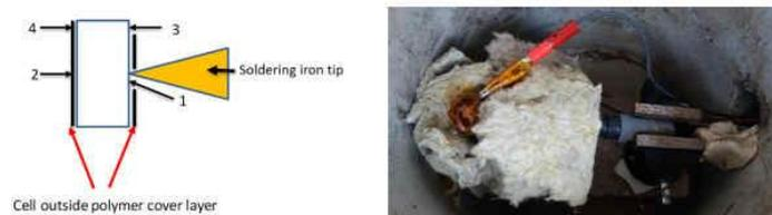
Figure 58: Thermocouple measurement points & setup insulation
