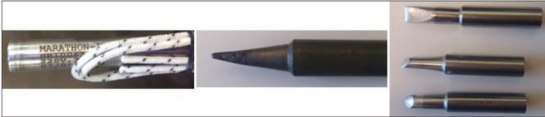
Figure 3: (Left) generation I cylindrical heating element, (Middle) generation II small area point contact tip, and (Right) various larger area point contacts with tip geometries selected for the geometry of the test cell casing.
