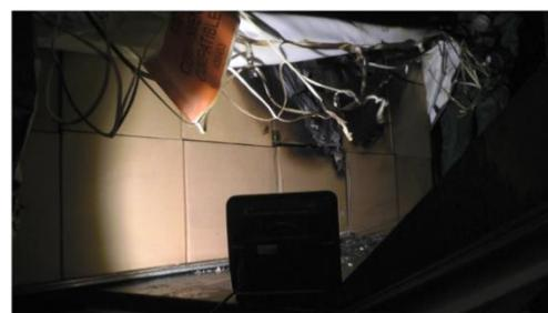
Figure 48: Fire Containment Cover after the test
