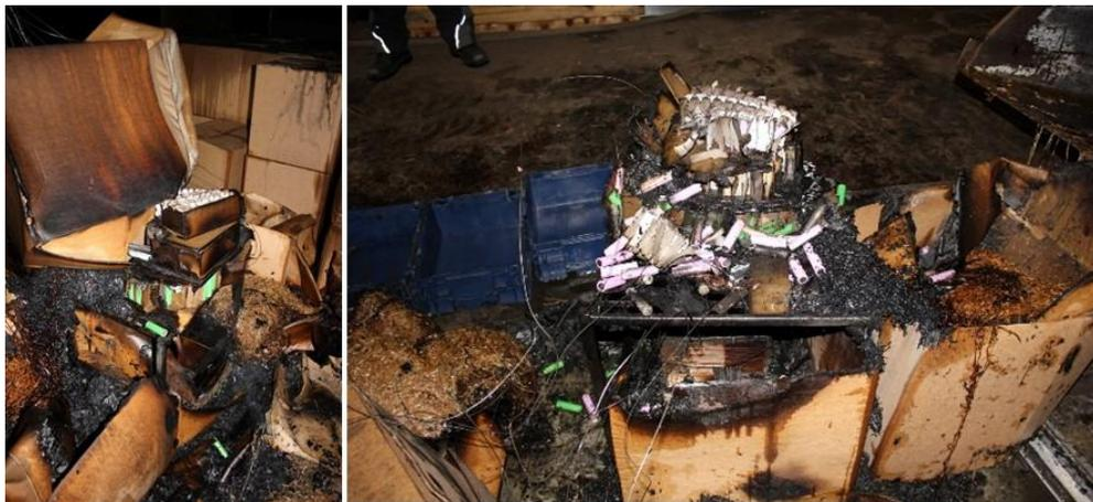
Figure 43: Impact on Cells after the test without fire suppression
