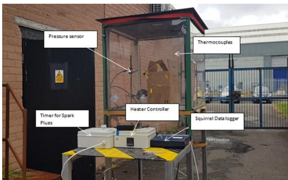
Figure 9: Test chamber built in accordance with SAE AS6413 Nov 2018 draft
