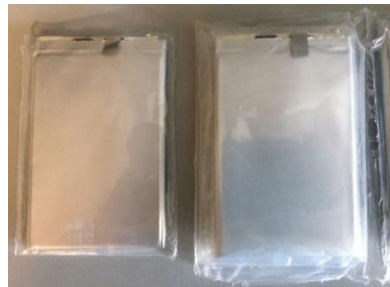
Figure 13: Lithium ion pouch cells: (left) cell individual wrapped in plastic envelope, (right) three such individually wrapped cells in secondary plastic envelope for redundancy. [Source: ALGOLiON Ltd.]
