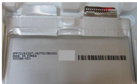
Figure 10: A pattern of holes and slots in a pouch cell tab (right side) acting as fuse. [Source: A123 Systems, Lt]
