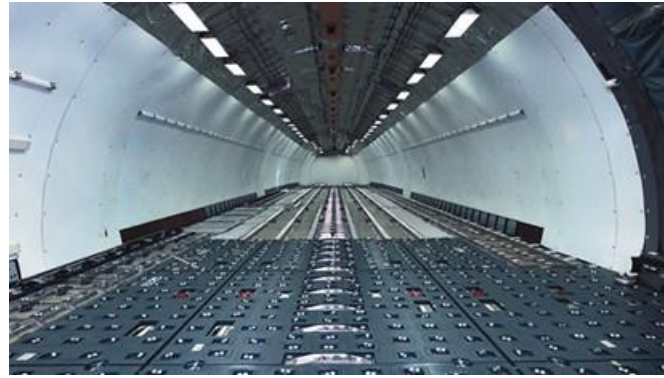
Figure 5: Class E compartment. [Source: The Boeing Company].
