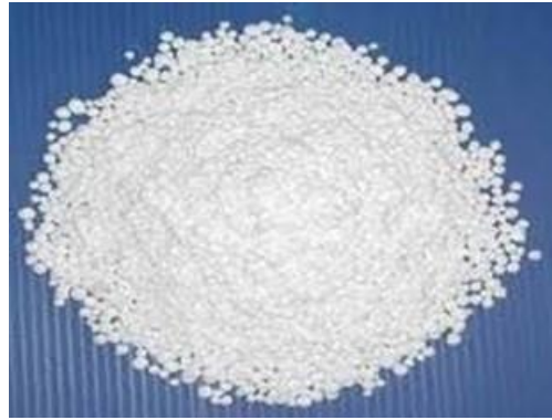
Figure 17: Paraffin wax is one type of PCM considered for lithium ion battery applications. [Source: Andores New Energy CO., Ltd., China].
