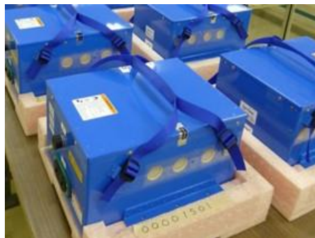
Figure 6: An example of a metal box required by the FAA to isolate the Boeing 787 Dreamliner operational batteries on-board the aircraft (there are two such units). [Source: The Boeing Company].
