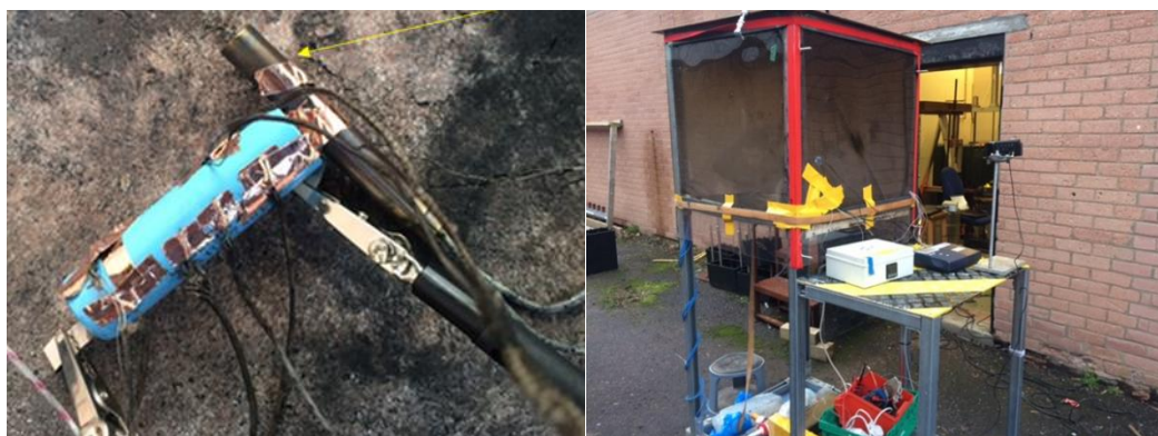
Figure 30: Left side – LG MH1 cell with heating element at base; Right side – heating test chamber at Impact Solutions.
