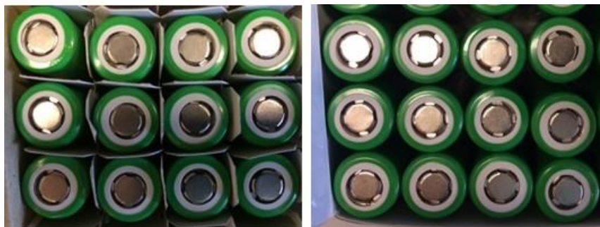
Figure 14: Lithium ion 18650 cylindrical cells: (left) cells packed with cardboard isolators between each cell, (right) cells packed with no isolators between them. [Source: ALGOLiON Ltd.]
